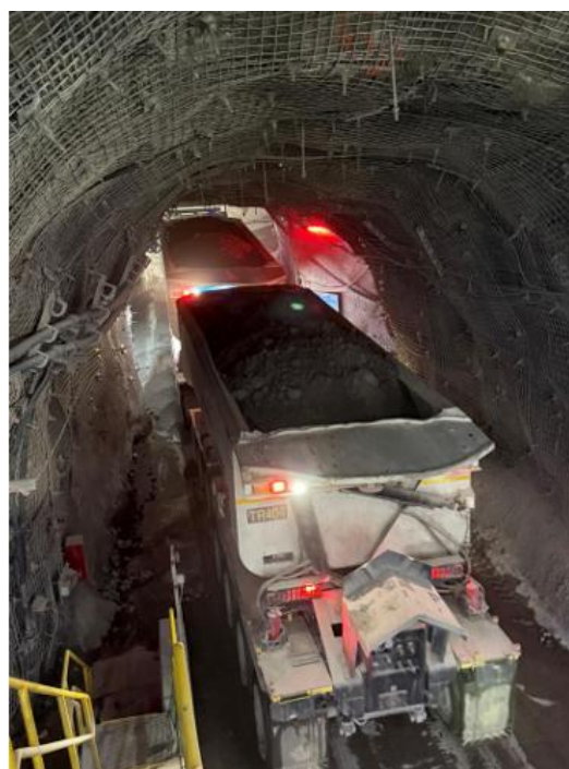
Road train delivering ore to underground crushers. Source: Entrée Resources – Sept 2026
